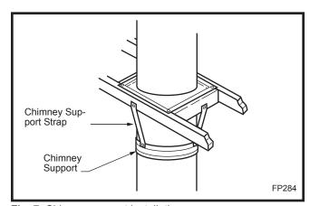
Fig. 7 Chimney support installation.
